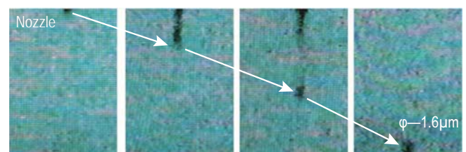
Photo 1 Observation of SIJ Droplet in Flight (For photography purposes, the droplet size was set larger than the standard size fired)
